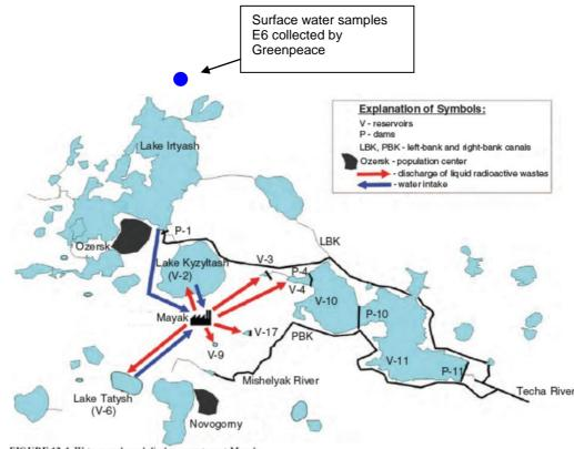
FIGURE 12-1 Water supply and discharge system at Mayak.
