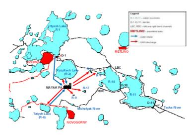
Fig.3 Layout of water use and liquid radioactive waste discharges from the Mayak PA
